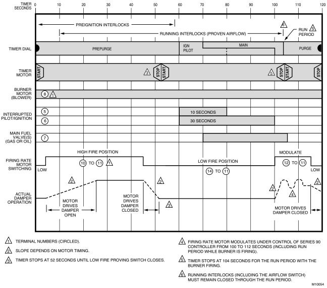
Fig. 4. Timer sequence for R4140G1015 Programmer.
